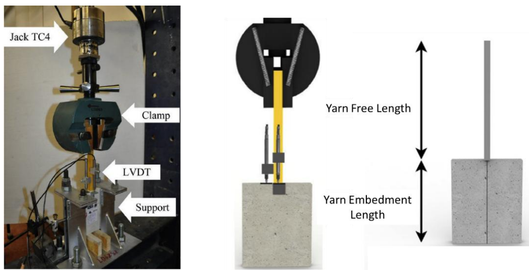
Figure 2-20 TRCC yarn pull-out test setup test setup (Dalalbashi et al., 2018)
