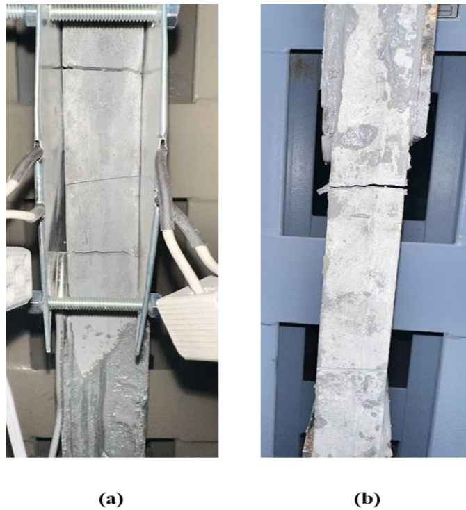
Figure 4-46 Cracking pattern in (a) 50°C,(b) 20°C
