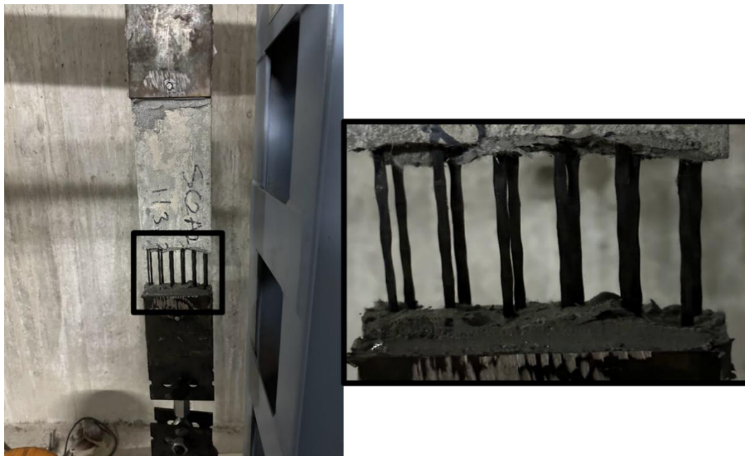
Figure 4-39 Pull out of carbon textile yarns in dummy specimens at 75% loading
