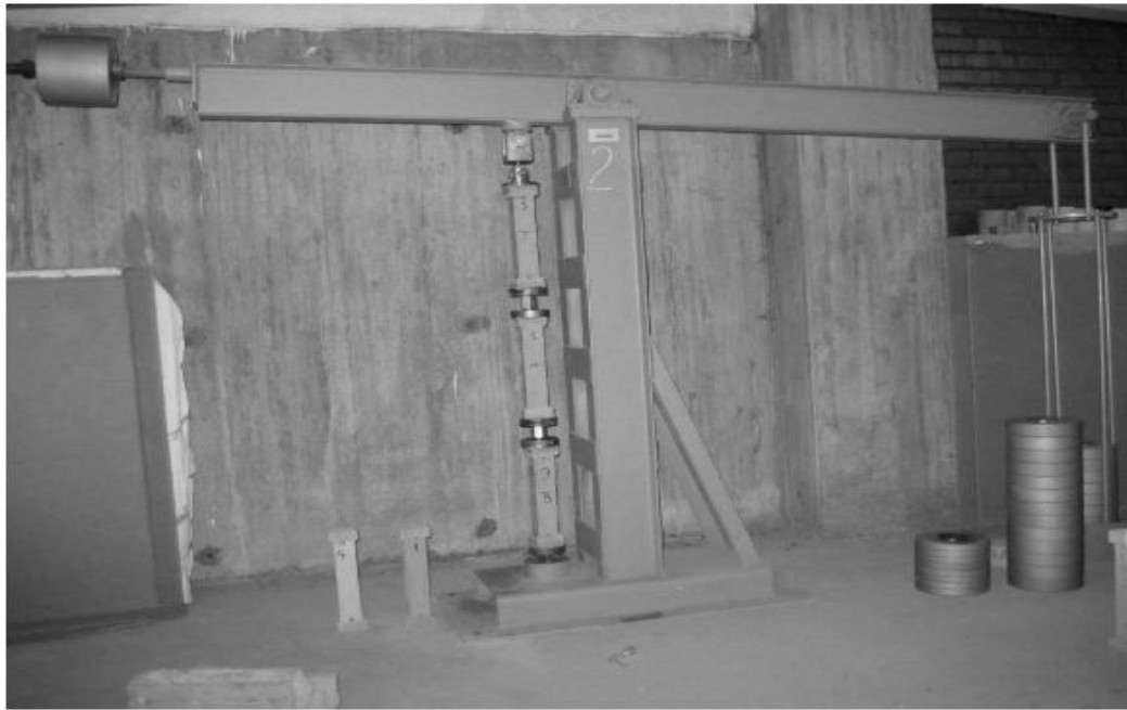
Figure 2-32 Tensile creep testing frame at METU (Keskin, 2012a)
