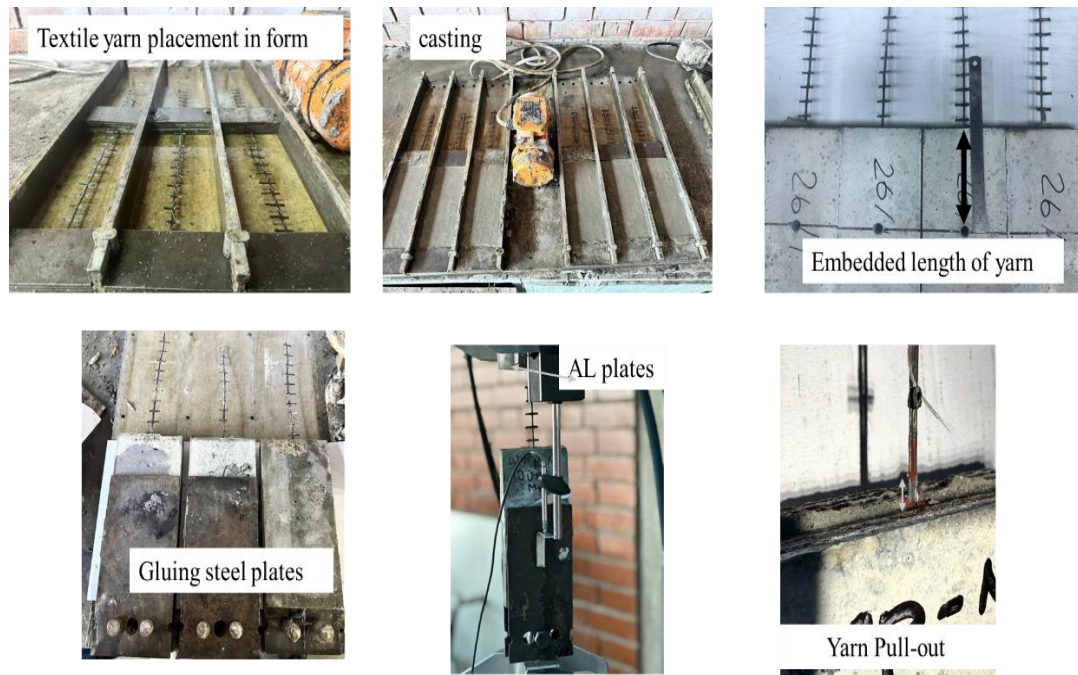
Figure 3-18 C-TRCC yarn pull-out tests specimen preparation and testing procedure.
